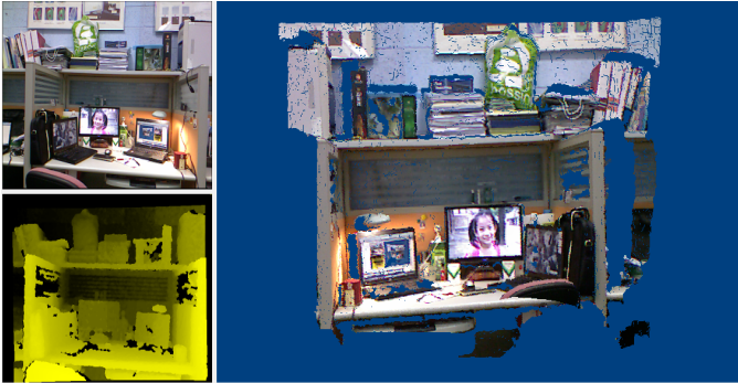
Figure 2. The color image (left-upper) and the depth image (left-lower) acquired by Kinect. (right) The colored cloud generated by incorporating every pixel in the color image with their corresponding depth value in the depth image.
